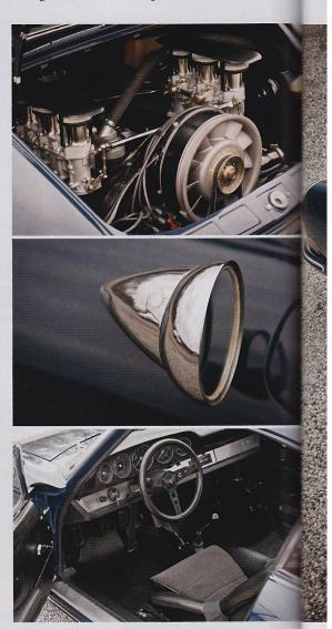
Amazingly the Aga Blue '67, which was outfitted as a competition car for Trans-Am use, retains its original race-prepared engine that was built on a '67 standard 901/06 engine case. Talbot mirrors were factory installed on both front fenders instead of the typical door-mounted mirror. The dash and gauges are original to the car and have likely never been removed. The odometer reads 17,479 miles.
