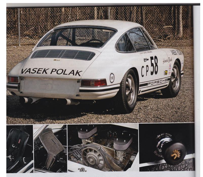
with the Webasto gas heater. Perhaps the most important components of the Rallye-Kit were the engine modifications comprised of polishing and port matching of the intake manifolds and cylinder heads, a competition clutch, special spark plug caps, and a special alternator.
