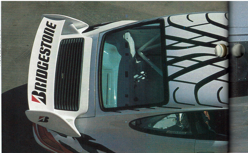
■ The five position adjustable rear wing is set at maximum downforce angle.
